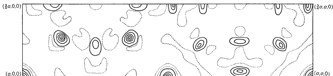
Fig. 4. Final difference Fourier synthesis of 4 × a 0 superstructure projected onto the (001) plane, with the displacement of uranium atoms taken into account (compare with Fig. 3).
